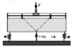
**Fig. 3c:** a set-up which might lead to a stress which propagates "along two lines": the pile is contained in a rigid container; the 2 soft springs ensure the equilibrium of the system, but most of the weight is carried by a rigid balance located in the middle which applies the force F+Mg-2 $\epsilon$ . Increasing the force F on top applies on the two pistons a force F/2 which is transmitted directly to the scales below, through the granular medium.
