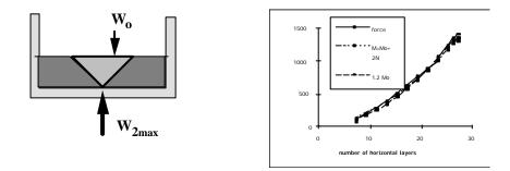
**Figure 5: Fig. 5a:** sketch of the experiment with a rectangular pile subject to different loads. The pile is stable as far as the bottom force does not exceed a given value  $W_{2max}$ , which depends on the pile height N and on the overload  $W_0$ . When  $W_2$  reaches  $W_{2max}$ , a finite deformation occurs in two zones inclined at 30° from vertical and the triangle moves up. The motion is a fraction of the grain diameter and leads to a diminution of  $W_2$ .
