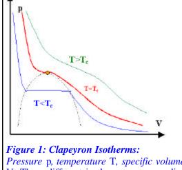
*Pressure* p, *temperature* T, *specific volume* V. Three different isotherms corresponding to Eq. (3). The green one corresponds to
