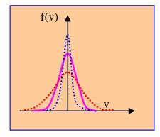
**Figure 3:** Local distribution of the speeds of particles in the model of § - 4.b. The three curves represent various places, at different temperatures of gas (blue at the cell centre, purple at a distance of a quarter cell from the wall, red in the edge). The distribution which dominates in high speed is the broadest corresponding to the highest temperature.
