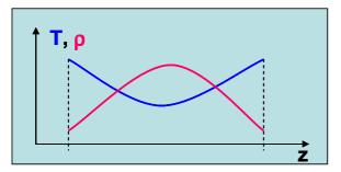
**Figure 2:** Temperature and the particle distributions in the cell containing a gas in thermodynamics equilibrium and evolving according to the model of § - 4.b, that is in which one extracts locally a heat proportional to the local energy of the local collisions
