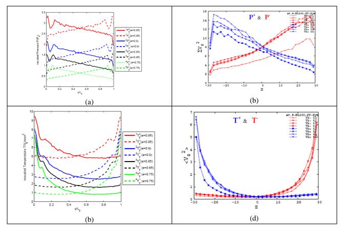
**Figure 6:** (a,b) Pressure  $P_+$  et  $P_-$  distribution in the cell as functions of the z position; they vary symmetrically with the distance to the excitation. Saw-teeth excitation. (a) : 2d case. (b): 3d cas. (c,d) temperature  $T_+$  et  $T_-$  distribution as functions of the z position; they vary symmetrically with the distance to the excitation. (c) : 2d case. (d): 3d case. [2,4,13.b]
